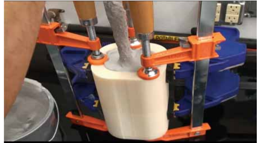
Forming sacrificial core in mold.
