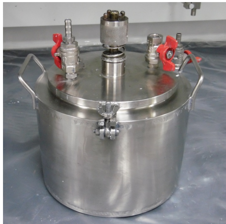
Enclosed Vessel with Vacuum and Nitrogen inlets
