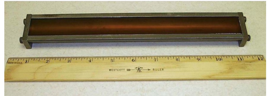
Linear Shrink Mold with Uncured Conventional UPR
