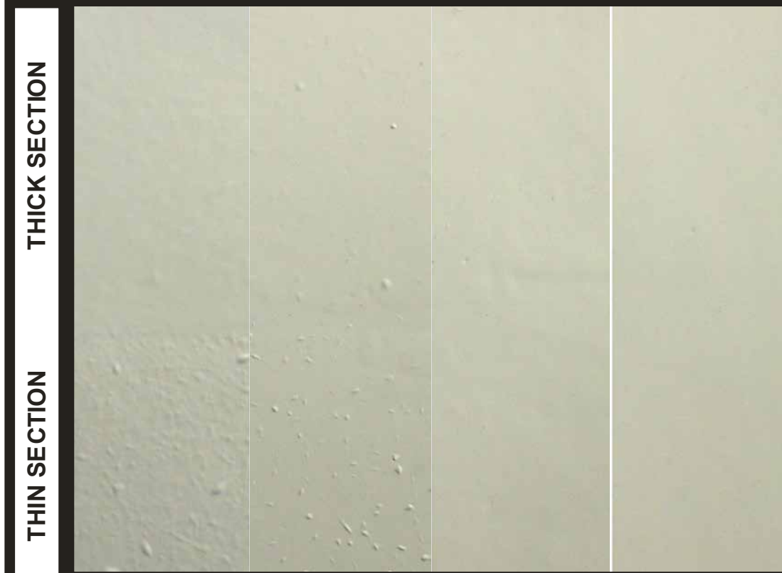
NO BARRIER VE SKIN with FIBER VE BARRIER BARRIER + SKIN
