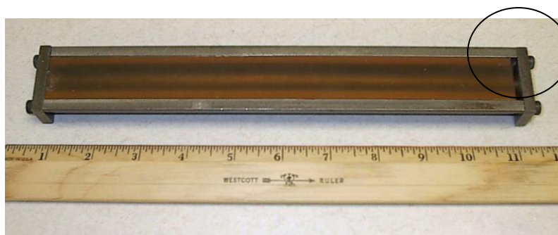
Linear Shrink Mold with Cured Conventional UPR
