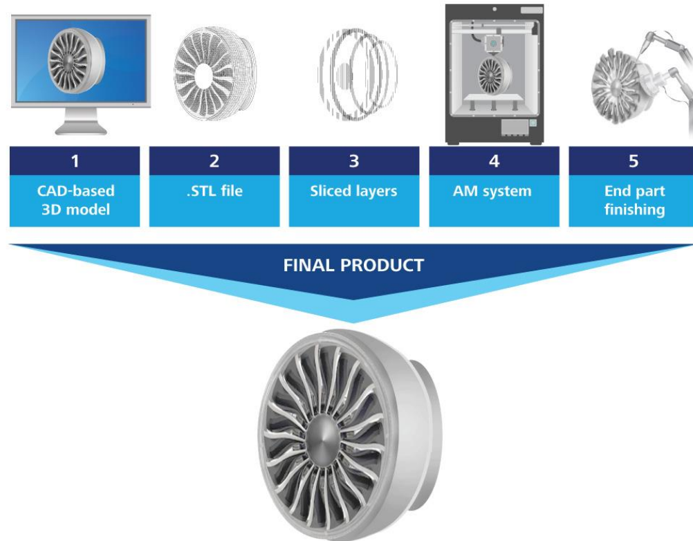
Figure 1. Additive manufacturing (AM) process flow
